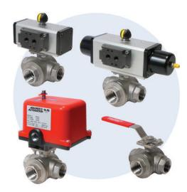
The 33D is a full port, 3-way, 316 stainless steel, NPT threaded end multi port ball valve. It can be equipped with a manual handle or with direct mount pneumatic or electric actuators. The direct mount actuators eliminate the valve-actuator mounting kit, which adds unnecessary height and expense.
