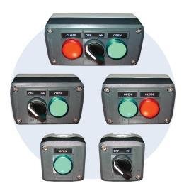
CB Series weatherproof control boxes allow the user to operate Assured Automation electric or pneumatic actuators from a remote location (pneumatic actuators require a solenoid). These compact control boxes are available with lamp indication for feedback confirmation of actuator/valve position (limit switch required).
