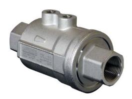
The VA and VIP Series combine a pneumatic actuator and valve into one body, eliminating packing glands, actuators and mounting kits. There are no exposed moving parts, eliminating pinch points and increasing operator safety. Since the actuator is part of the valve, costs are greatly reduced when compared to standard actuated valves.
