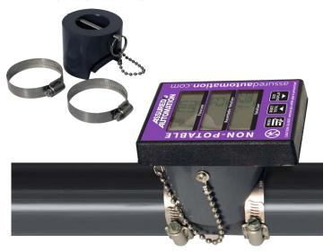
**Saddle Mount:** the meter comes with a "saddle" and 2 hose clamps that are used to attach the meter to an existing pipe. Once the saddle is attached to the pipe, a hole must be drilled in it for the paddle wheel to enter the pipe through.
