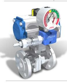
The TSV series Thermal Shut-off valves combine a fire-safe ball or butterfly valve with a pneumatic actuator and the **FM approved** *FireChek®* valve to form a dedicated stand-alone thermal shut-off valve that will close (or open) at a given temperature (165° F standard). This alternative to fusible link valves can be tested and reset without the need to replace any hardware.
